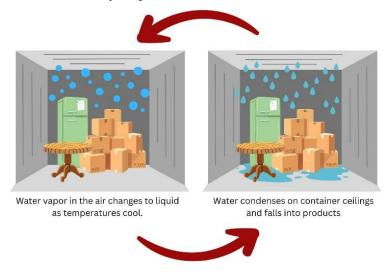
A certain amount of moisture vapor is naturally in the air and when the temperature drops, it creates condensation. If the temperature drops below the dew point, water droplets form. As the container sweats and temperatures rise, the moisture collects and essentially "rains" inside the unit/container.
